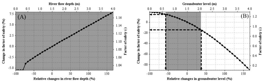
**Figure 4. Simulated bank stability (factor of safety) as a function of variations in a range of hydrological parameters. (A) River water level, and (B) groundwater table.**
