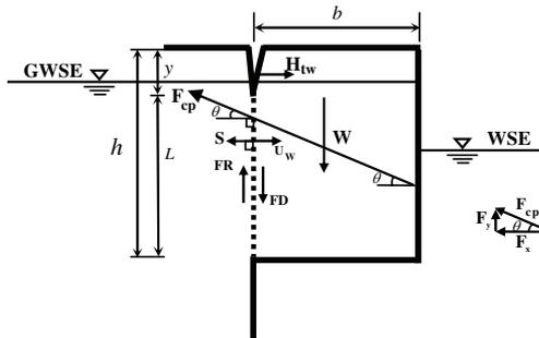
**Figure 1. The bank geometry and forces exerted on the incipient failure block.**
