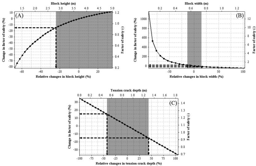
**Figure 2. Simulated bank stability (factor of safety) as a function of variations in a range of bank geometry parameters. (A) Block height, (B) block width, and (C) tension crack depth for the reference block used in the sensitivity analyses (see Table 1 for definition of the reference block).**
