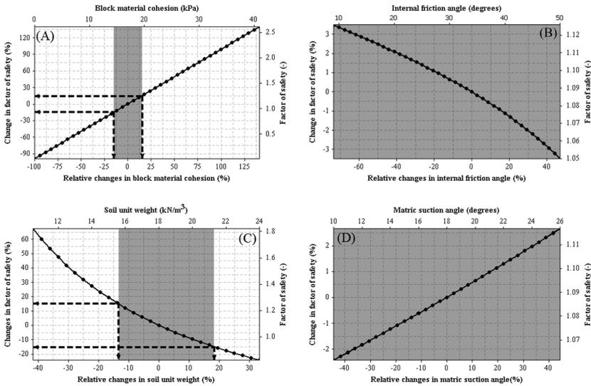
**Figure 3. Simulated bank stability (factor of safety) as a function of variations in a range of geotechnical parameters. (A) Soil cohesion, (B) soil friction angle, (C) soil unit weight, and (D) matric suction angle.**
