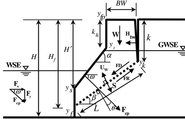
**Fig 1:** The bank geometry and forces exerted on the incipient failure block
