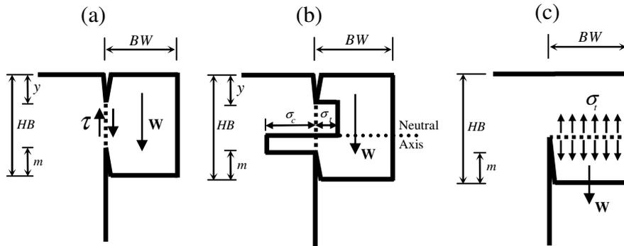
**Fig 3:** Forces of weight, shear, compression and tension acting on a cantilever with regard to the three modes of failure: a) Shear failure; b) Beam failure; c) Tensile failure. (From Thorne and Tovey, 1981)
