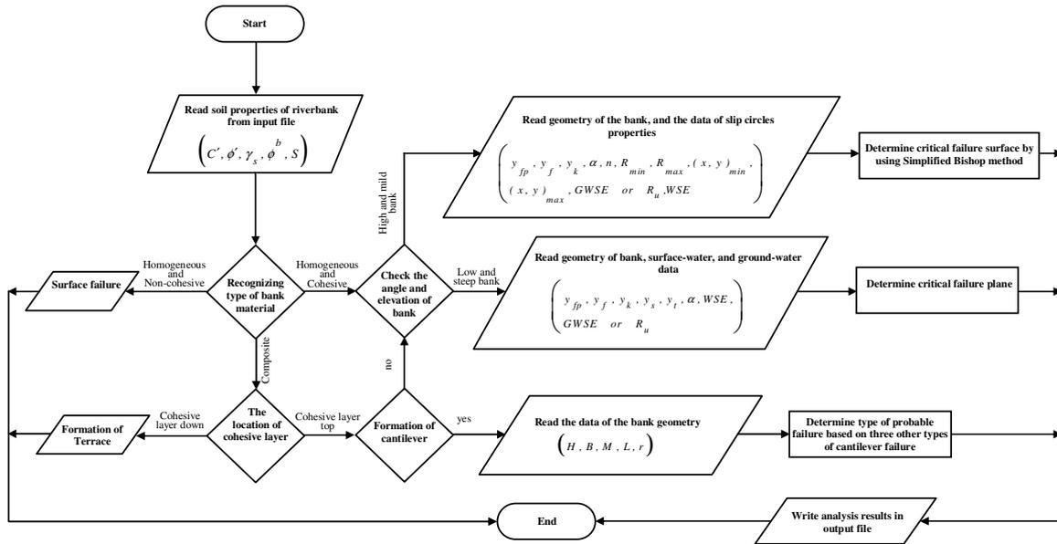
**Fig 4:** Diagram illustrating the computational procedure employed in EMSAR.
